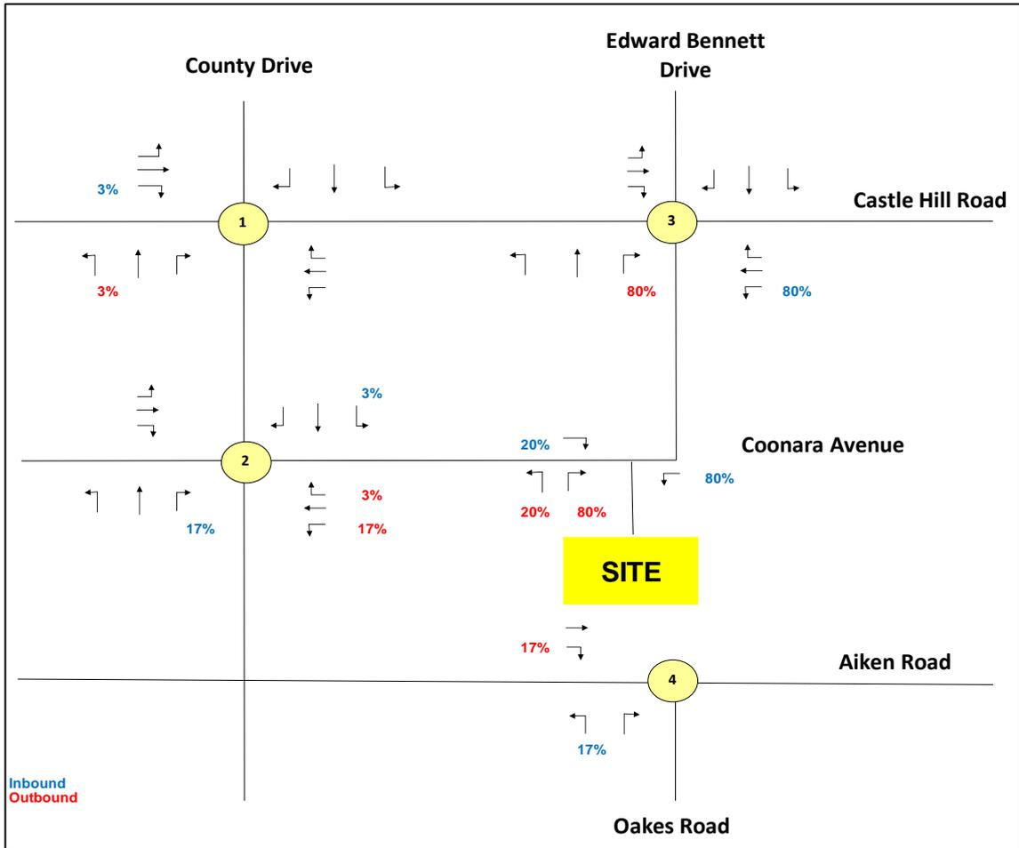
Additional traffic generated due to the development under Scenario 1 is shown in Figure 3.2 for the AM peak hour and Figure 3.3 for the PM peak hour.
