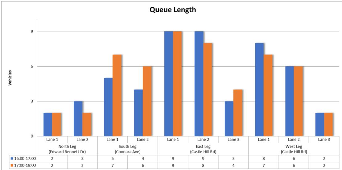
Figure 2.12: Observed Queue Length at Highs Road/ Castle Hill Road/ County Drive intersection
