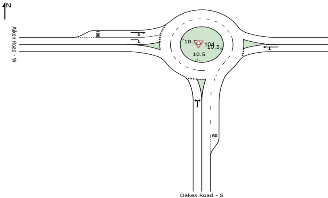
The dual right turn provides additional storage capacity and the SIDRA results illustrate that the intersection performs at LOS B and has a DOS of 0.85. Detailed SIDRA results are provided in Appendix B.
