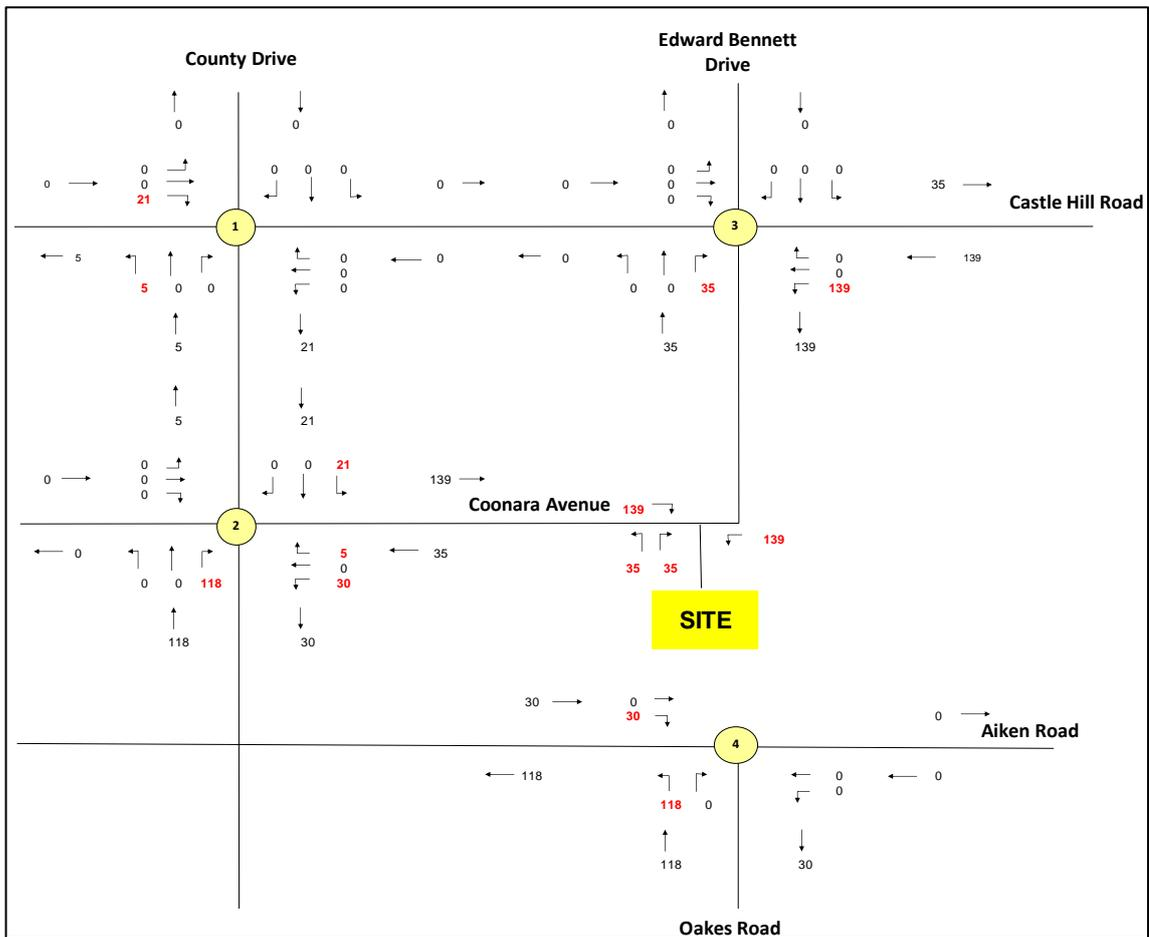
Total traffic with the proposed development under Scenario 2 is shown in Figure 3.14 and Figure 3.15 for AM and PM peak hours respectively.
