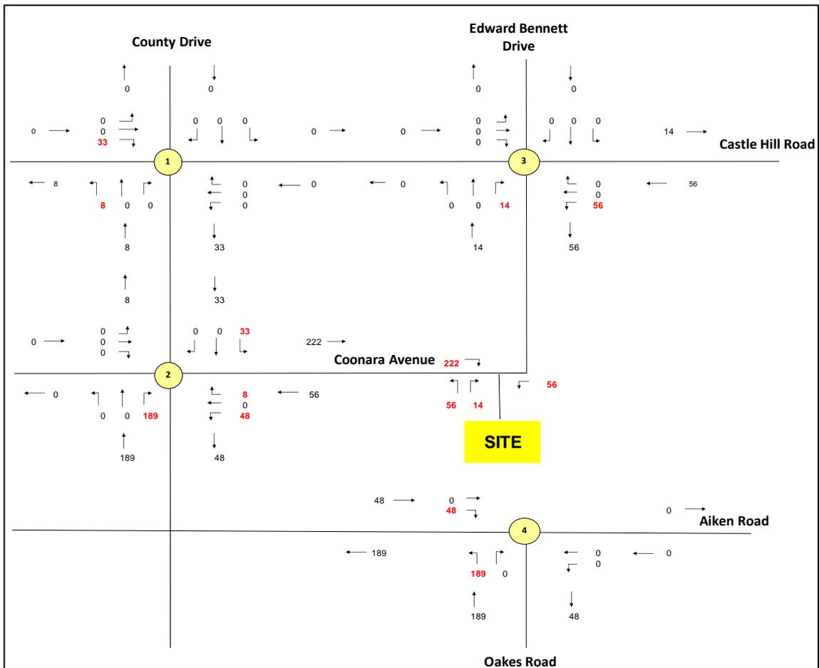
Total traffic with the proposed development under Scenario 2 is shown in Figure 3.9 and Figure 3.10 for AM and PM peak hours respectively.
